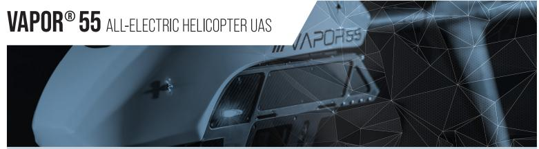
The all-electric VAPOR 55 Helicopter UAS delivers flight control performance, endurance, and payload flexibility. Featuring military-grade components, intelligent HW/SW system design, and high energy density lithium-polymer battery, VAPOR delivers enhanced flight stability and up to one hour of flight time on a single battery charge.
