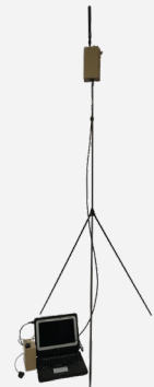
FIRE CONTROL SYSTEM WITH TABLET CONTROLLER
