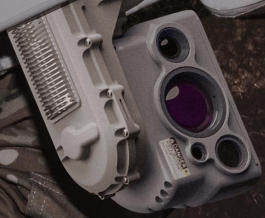
A close-up photograph of a Mantis imaging payload sensor mounted on a white aircraft fuselage. The sensor is a compact, grey, rectangular unit with a prominent lens and several smaller circular ports. It is secured with a metal bracket. The background shows a person in military camouflage gear and a dark, wooded area.
