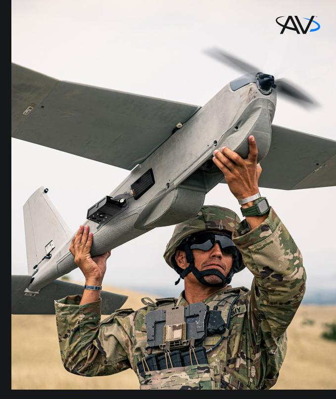
AV's Puma™ VNS is a visual-based navigation system for Puma 2AE, Puma 3AE, and Puma LE small unmanned aircraft systems (SUAS). Puma VNS enables GNSS-denied navigation across GNSS-contested environments. The system performs Visual Inertial Odometry (VIO) through a suite of integrated sensors and an onboard compute module to determine the precise location of the aircraft during flight.
