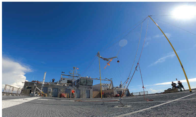
Puma 3 AE is recovered by the Precision Recovery System while USNS Carson City is underway during REP(MUS) 21. Photo credit: AeroVironment, Sept. 2021.
