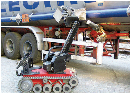
tEODor EVO secures a chemical pipe access port in this training scenario.
