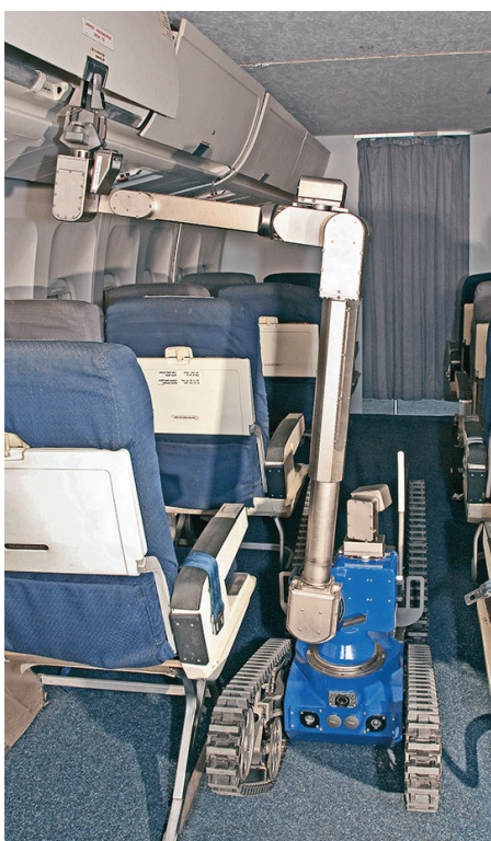
The telemex EVO Hybrid opens an overhead bin during an airplane training scenario.
