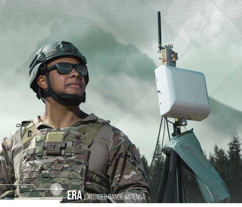
The ERA is a lightweight, portable antenna array kit designed to integrate seamlessly with AeroVironment's Standard Range Antenna to support a diverse range of missions. The ERA add-on kit narrows the antenna beam width, extending the command and control range up to 40 kilometers (24.9 miles) or 100 percent greater controllable range over the Standard Range Antenna with minimal impact to its size, weight and power (SWAP) footprint.
