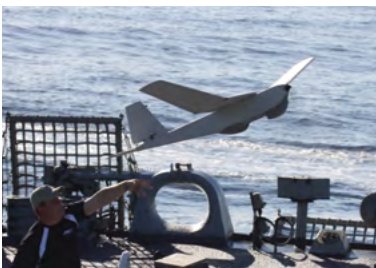
Puma is launched from a ship
