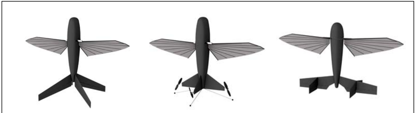
Various airframe configurations similar to those used in the early Phase I effort to begin investigating control system effectiveness, prior to the tailless design.
